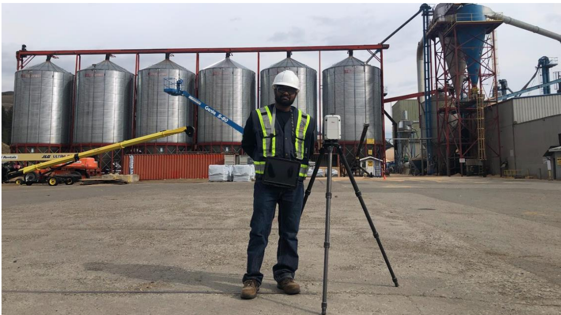
Prashanth using Leica 3D scanner to capture site data at Princeton BC
