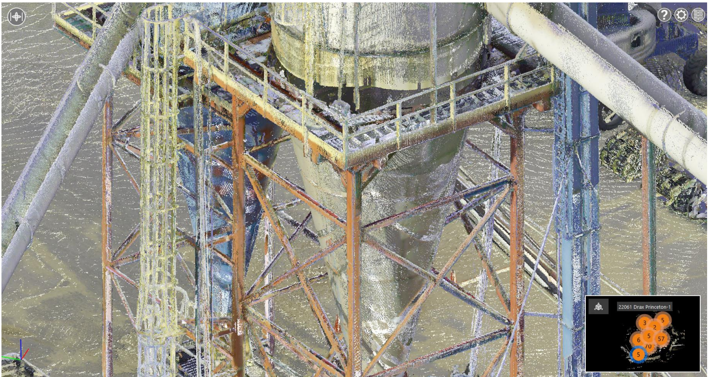
3D Scan of the plant stitched together in top view (Zoom into structural steel support)
