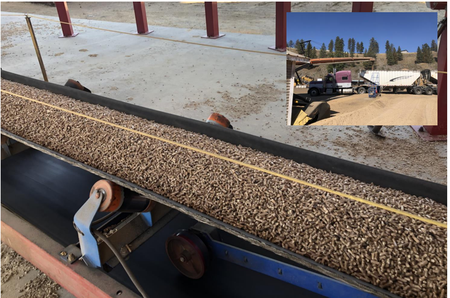
Wood pellets being produced in Princeton BC and getting loadout using belt conveyor to fill truck
