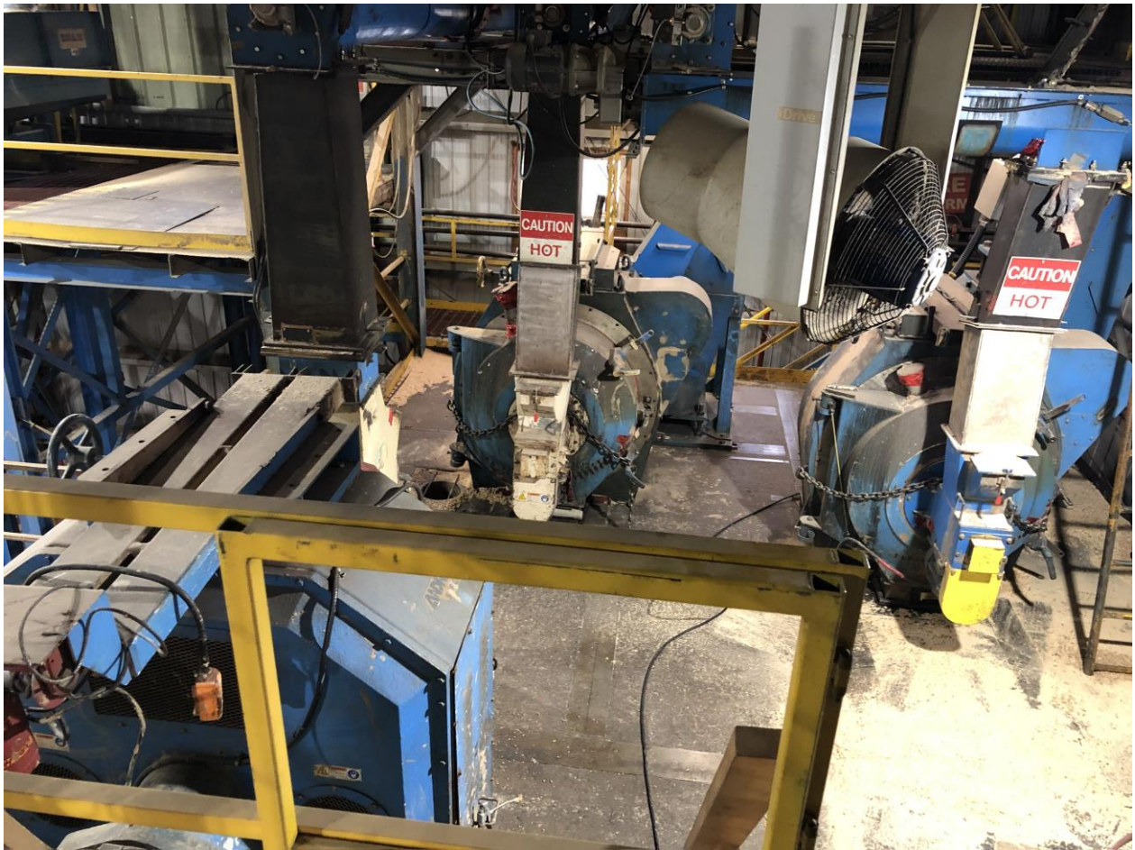
Pelletizers layout on structural steel platform
