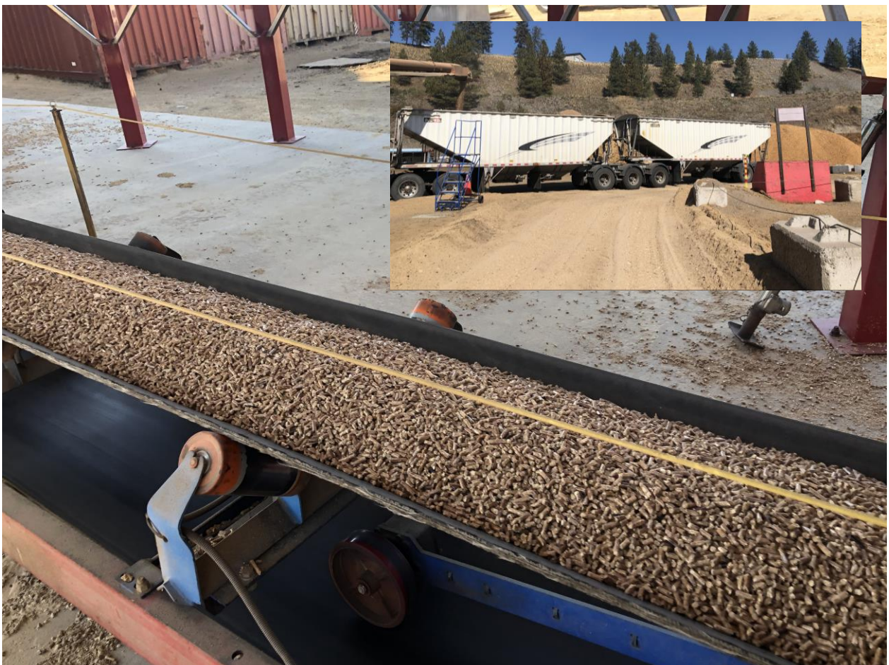
Pellets on belt conveyor under the storage silos loading into a truck
