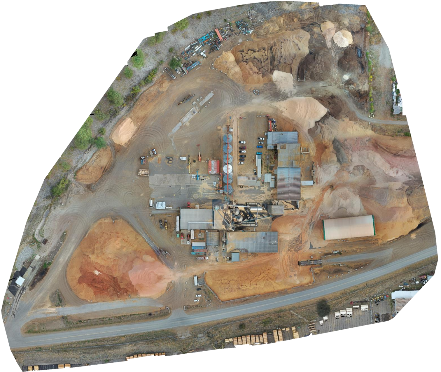
Orthomosaic of the Princeton BC pellet plant: This orthomosaic is composed of 426 photos stitched together
