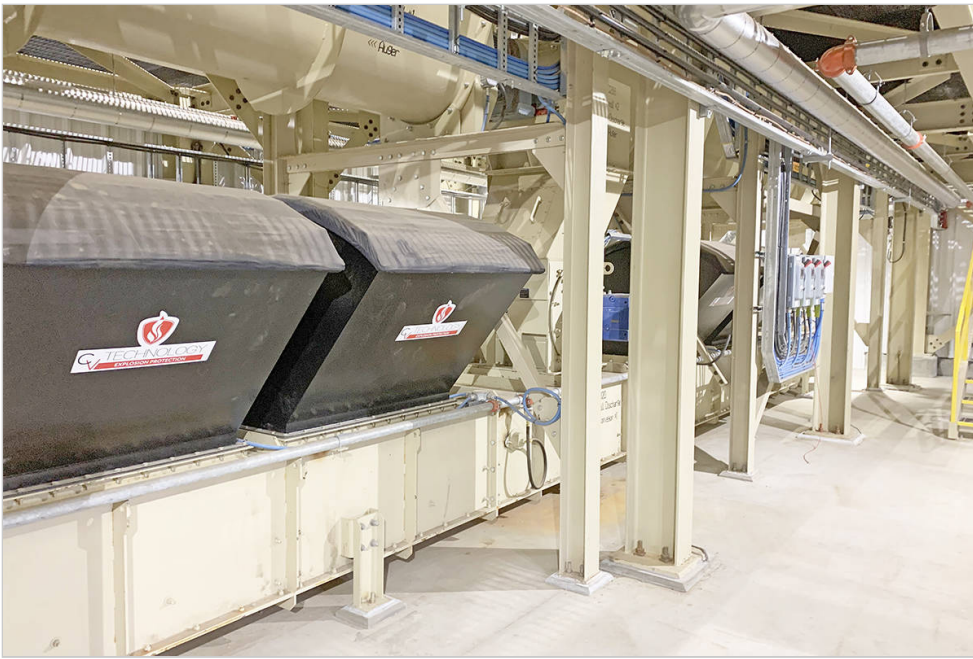
Flameless vents are part of the new addition at Pinnacle Renewable Energy in Williams Lake. (photo submitted)
