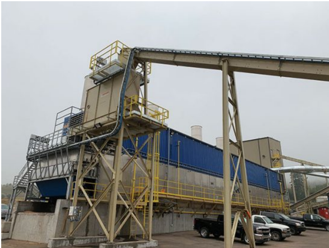
A view of the bed dryer infeed at Pinnacle's Williams Lake, B.C. plant, showing the infeed conveyor and metering bin supplied by Continental Conveyors. Photos courtesy Pinnacle Renewable Energy.
